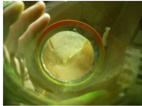
Cut and carefully place/seal coffee filter as the first "membrane"
